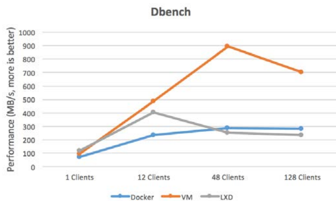
Fig. 5. Performance results for I/O for varying number of parallel client processes under Dbench benchmark
